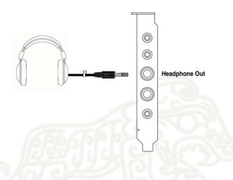
The Headphone Out port has a built-in high-quality amplifier for headphones. Connect your stereo headphones to the headphone output ports on the Xonar Essence ST card.
